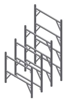
The HI-LITE 12K aluminum shoring frame system has a capacity of up to 53.4 Kn (12,000 lb.) per leg using a safety factor of 2.5.
