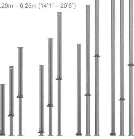
The all-new **HI-LITE H-MAX** (The Maximum Series) is a one-piece aluminum post shore with a captured aluminum screw jack. All HI-LITE products incorporate our signature feature of the continuous T-Bolt slot, allowing for the addition of many accessories such as gates and cross braces to assemble the post shores into towers.
